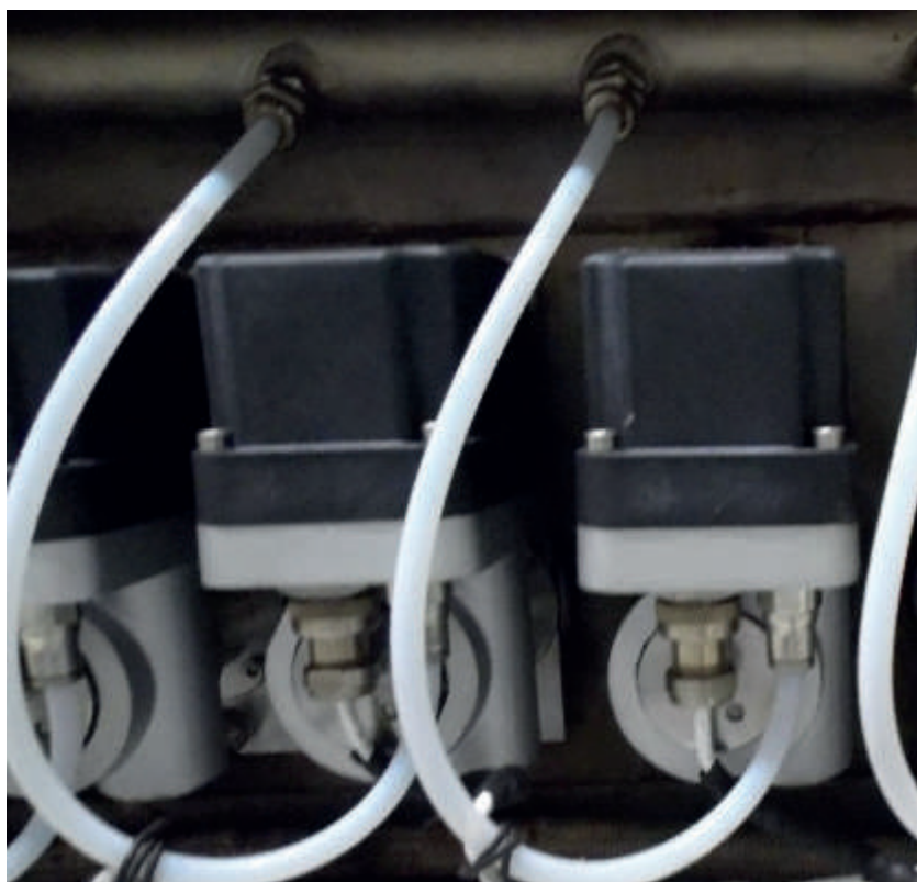
Figure 6. New Tasowheel STA-1015 actuators.
